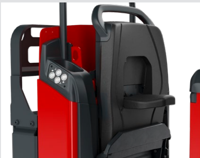
Adjustable backrest with foldable operator's seat
